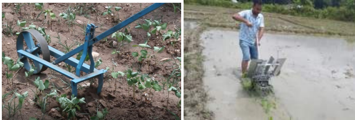
Image: Wheel hoe on left, Paddy transplanter on right
