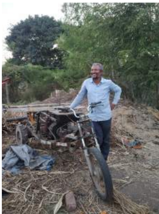
Image: 'Sanedo' transformed into mini tractor by attaching various attachments. This is used for land preparation, sowing and weeding.
