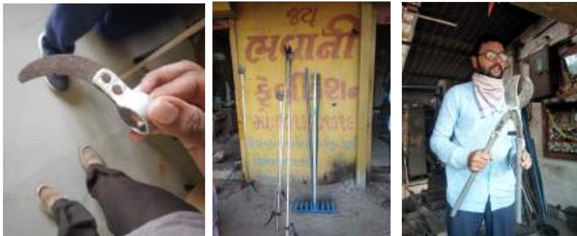
Image on the left: Bhindi plucker by Krish Vigyan Kendra, Sanosara, Bhavnagar. Image in middle: The scissors for drumstick made locally using cycle brakes. Image on the right: handmade replica of store available scissor.
